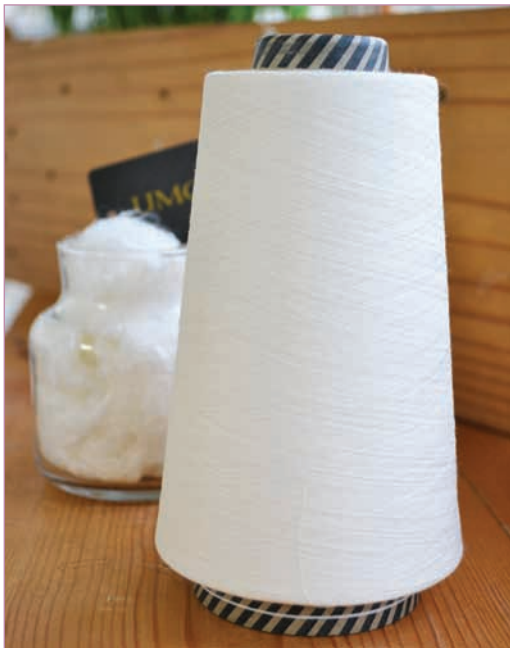
Umorfil Beauty Fiber, introduced by Camangi and used by weaver HerMin Textile and knitter Eclat, is the result of a nanotechnology used to integrate ocean collagen peptide sourced in Taiwan into polyester or viscose fibres.
